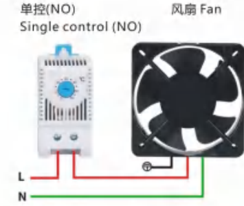
单控(NO)搭配风机接线图 Single control (NO) with fan wiring diagram
